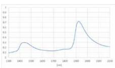
peak absorption wavelength by target substance can indicate an existence of substance. This sample shows that the water is contained by observing the absorption peak at 1450 and 1920nm.
