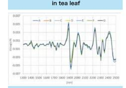
The second derivative of absorbance can compare the difference of absorption for each ingredient. This utilizes the absorption wavelength differs from ingredient. If the multiple ingredients intricately mixture, the mathematical method such as the multivariate analysis can be applied
